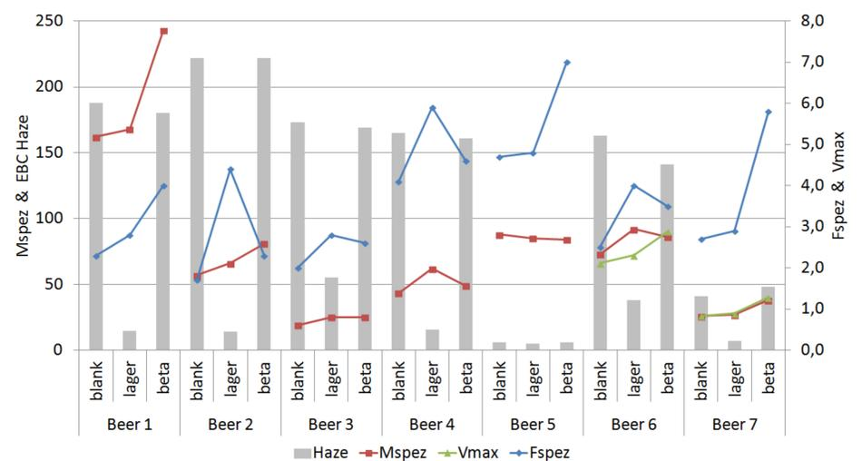
Precoat and membrane filtration flux rates usually change when beer is lagered/decanted or enzyme treated but these changes are not always significant. Sometimes flux rates of precoat and membrane mode react similar on treatments, sometimes not. This is not surprising and confirms, that it makes sense to model industrial scale filtration modes with equivalent modes at lab scale.
