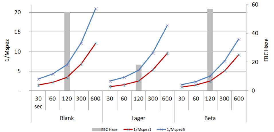
The tested Pils beer shows improved flux rates when beta-glucanase treated or lagered and decanted. Backflush efficiency of this beer is then also improved.
