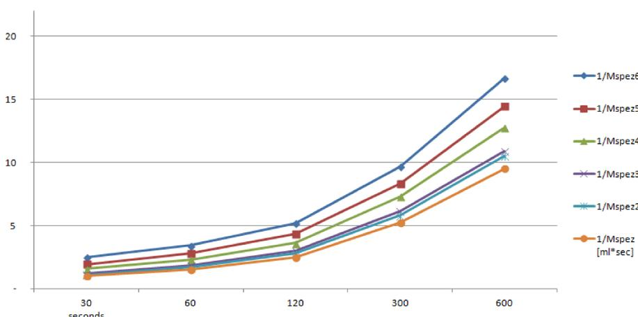
The inversed values of the flux rates (1/Mspez) are modelling pressure increase curves. Differences in pressure curves after backflushes could indicate backflush / cleaning efficiencies.
